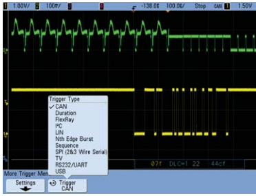
Trigger on and decode CAN serial packets.
